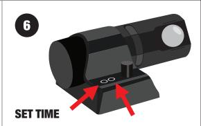
Push the button and the minute hand will move forward by one minute, hold the button and the minute hand will move forward rapidly.
