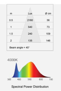
luminous flux, rated beam angle and rated wattage are equivalent to their nominal values shown on product packaging. There is no measurable output from 180nm to 380nm, so the chart shows only 380nm to 800nm.
