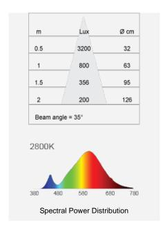
Remarks: The rated lamp life, rated luminous flux in 90  $^{\circ}$  cone, total luminous flux, rated beam angle and rated wattage are equivalent to their nominal values shown on product packaging. There is no measurable output from 180nm to 380nm, so the chart shows only 380nm to 800nm.
