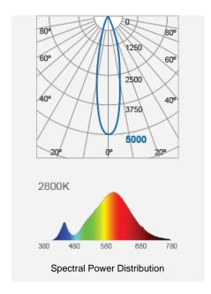
Remarks: The rated lamp life, rated luminous flux in 90  $^{\circ}$  cone, total luminous flux, rated beam angle and rated wattage are equivalent to their nominal values shown on product packaging. There is no measurable output from 180nm to 380nm, so the chart shows only 380nm to 800nm.
