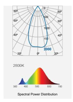
Remarks: The rated lamp life, rated luminous flux in 90 ° cone, total luminous flux, rated beam angle and rated wattage are equivalent to their nominal values shown on product packaging. There is no measurable output from 180nm to 380nm, so the chart shows only 380nm to 800nm.
