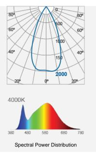
Remarks: The rated lamp life, rated luminous flux in 90 ° cone, total luminous flux, rated beam angle and rated wattage are equivalent to their nominal values shown on product packaging. There is no measurable output from 180nm to 380nm, so the chart shows only 380nm to 800nm.
